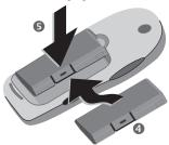
Insert cover in the lower edge 6, then press downwards 7, until it engages.
