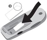
Insert battery into the phone sideways 4, then press downwards
