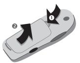
Insert SIM card in the opening with contacts pointing downwards and push gently until it engages (make sure the angled corner is in the correct position 3).
